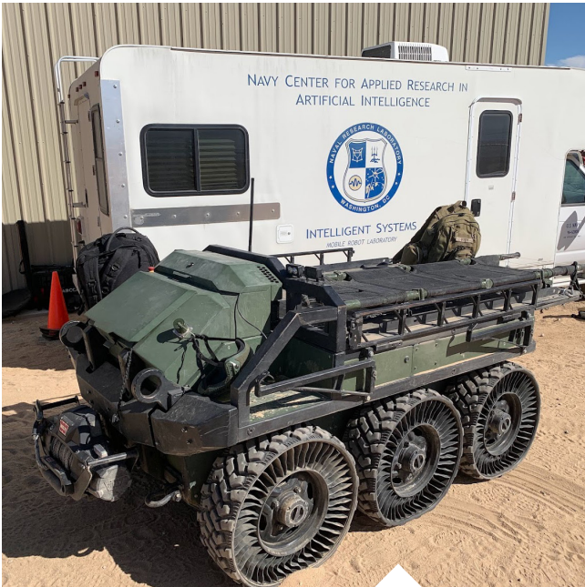
(Above) The Hunter WOLF, developed by HDT Expeditionary Systems, is prepared for arduous testing in real-world conditions at Range 220 onboard US Marine Corps Base Twentynine Palms. This project was created and led by LT ES Vorm, PhD from the US Naval Research Laboratory's Navy Center for Applied Research in Artificial Intelligence as part of a 6.5 funding activity to demonstrate and evaluate the concept of autonomous casualty evacuation.
