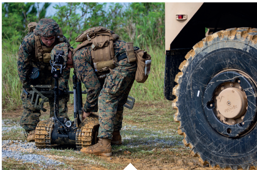
Staff Sgt. David Cain and Sgt. Maximilian Musick lift the tracks of the Mark II Talon explosive ordnance disposal robot during charge employment training Aug. 2, 2018 at Camp Hansen, Okinawa, Japan. The training taught EOD technicians to effectively neutralize IED threats with unmanned robotic platforms by safely finding and removing any hazards. Cain, a native of Fredericksburg, Virginia and Musick, a native of Phoenix, Arizona are EOD technicians with EOD Company, 9th Engineer Support Battalion, 3rd Marine Logistics Group. (U.S. Marine Corps photo by Pfc. Terry Wong)
