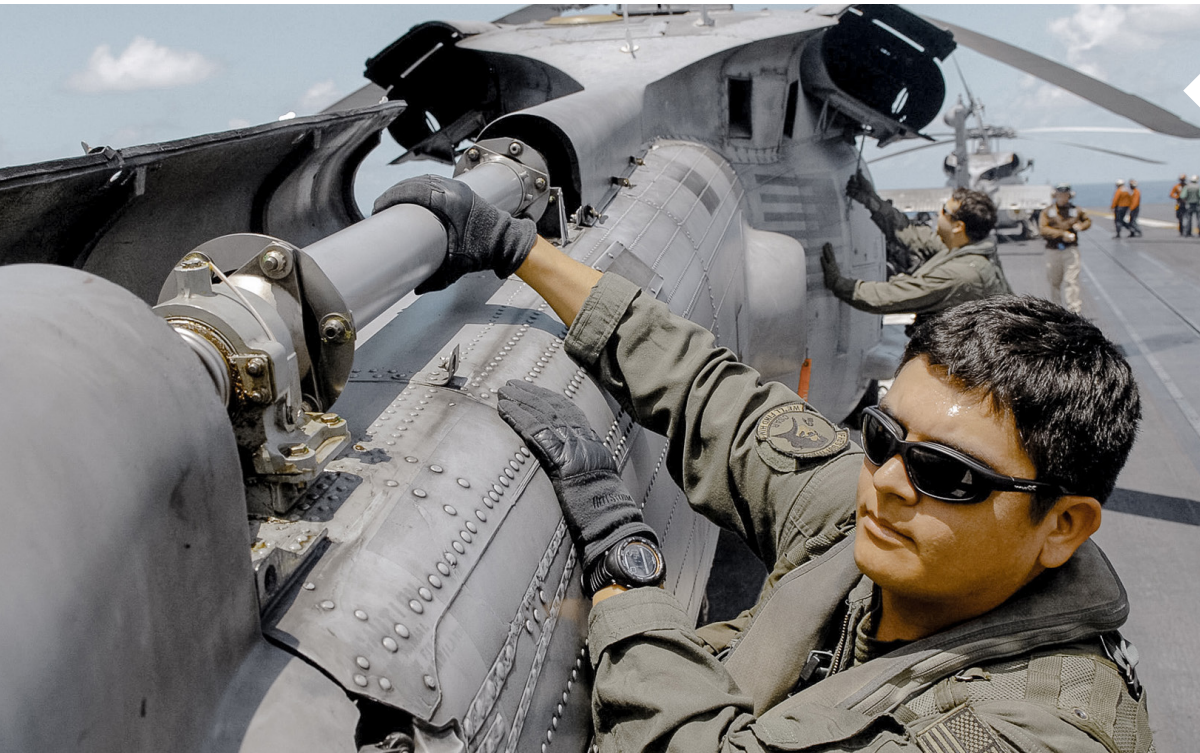
Petty Officer 2nd Class Vincent Rodriguez inspects the tail rotor drive shaft as he performs a preflight check on an H-60H Seahawk helicopter on the aircraft carrier USS Abraham Lincoln (CVN 72) as the ship operates in the Pacific Ocean. Photo by Petty Officer 2nd Class James R. Evans, U.S. Navy
