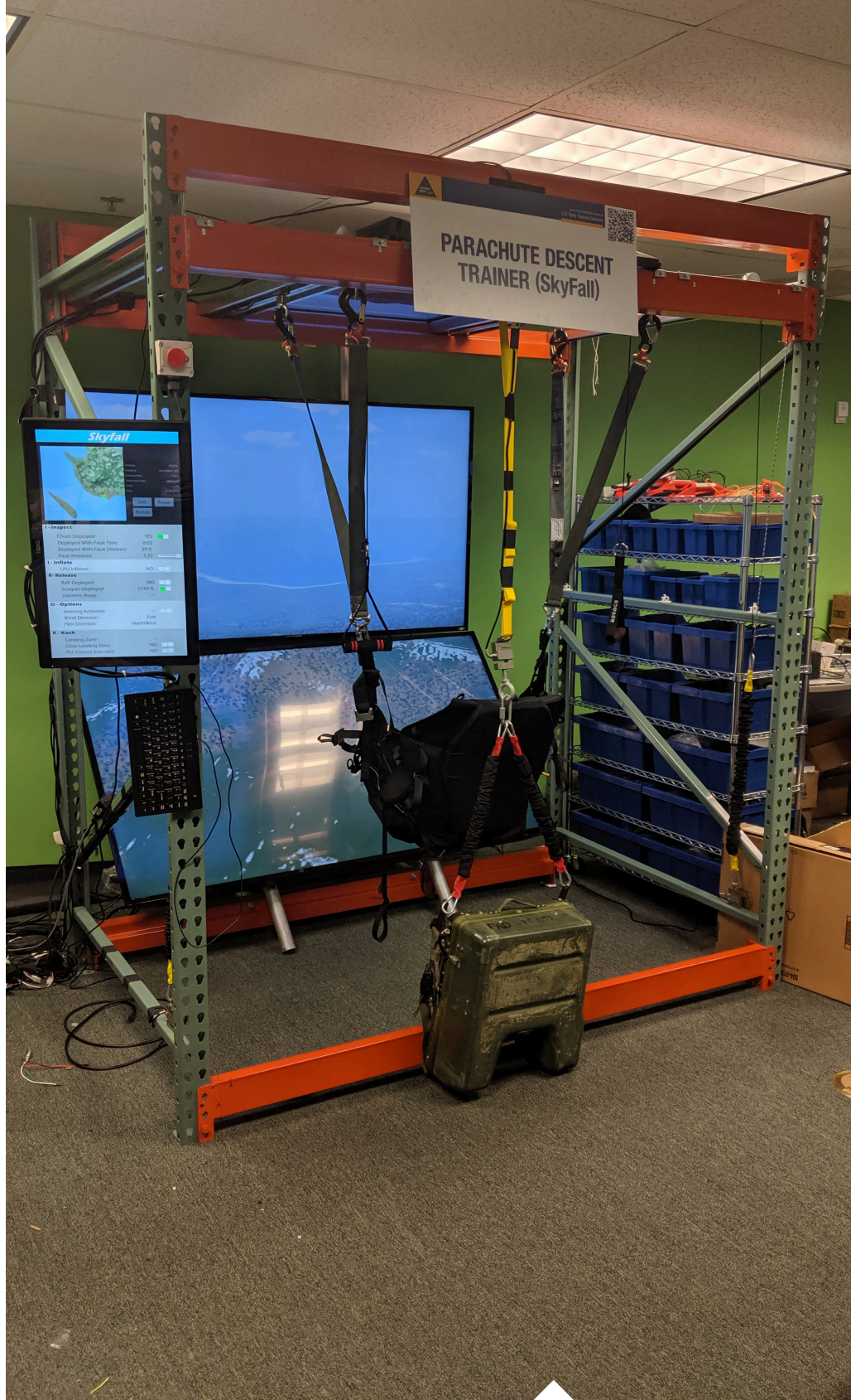
Above: The parachute descent trainer prototype, currently undergoing user testing and evaluation at locations in Pensacola, Florida and Lemoore, California
