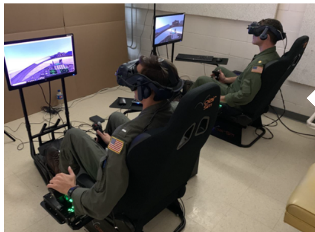
Left: A MR T-45C Goshawk Jet merging a simulator cockpit with a virtual environment, was created by BISim and integrated with the 2F138D Operational Flight Trainer (OFT) at NAS Kingsville. This system is called the Augmented Reality Visual System (ARVS) and leveraged a Varjo HMD.
