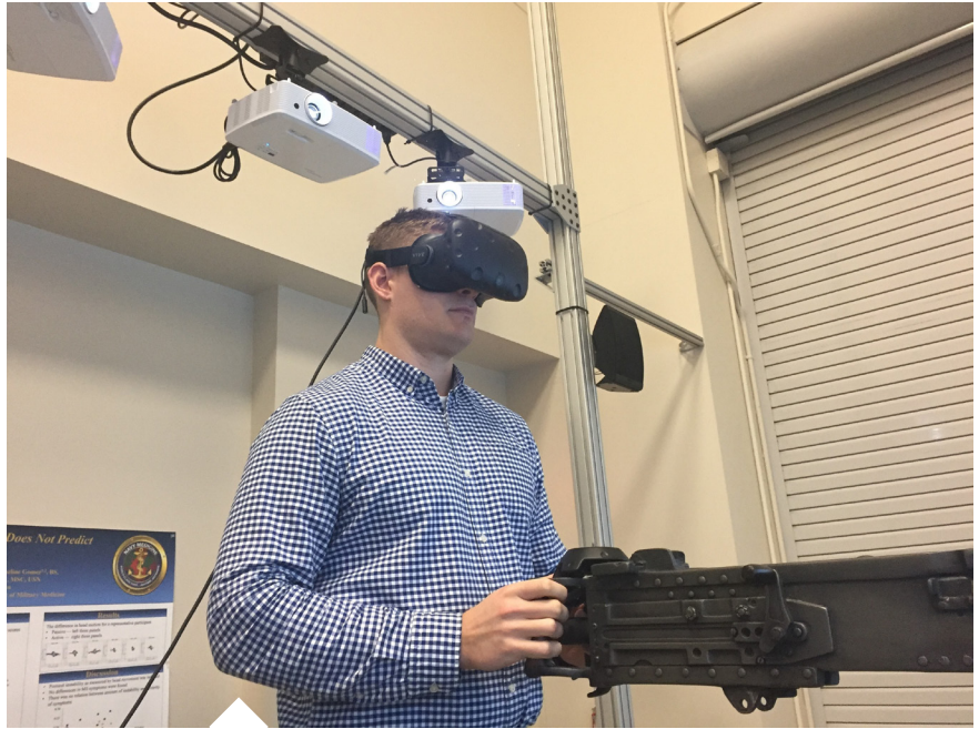
Above: A mixed reality system simulates the motion of a US Navy Destroyer in order to study the effects of subtle motion on object tracking and accuracy tasks. In this study, a participant is given targets at which to fire a simulated M2 Browning Machine Gun.
