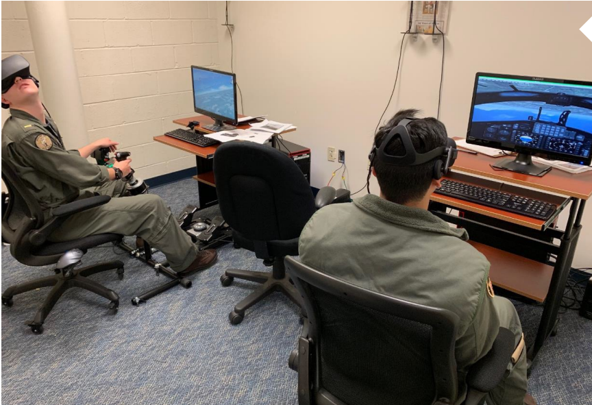
Left: Two flight students at Naval Air Warfare Center, Training Systems Division in Orlando, FL use the VR-Part Task Trainer (PTT), learning to operate a T-45C Goshawk jet using Oculus Rift head mounted displays and Prepar3D simulation software.
