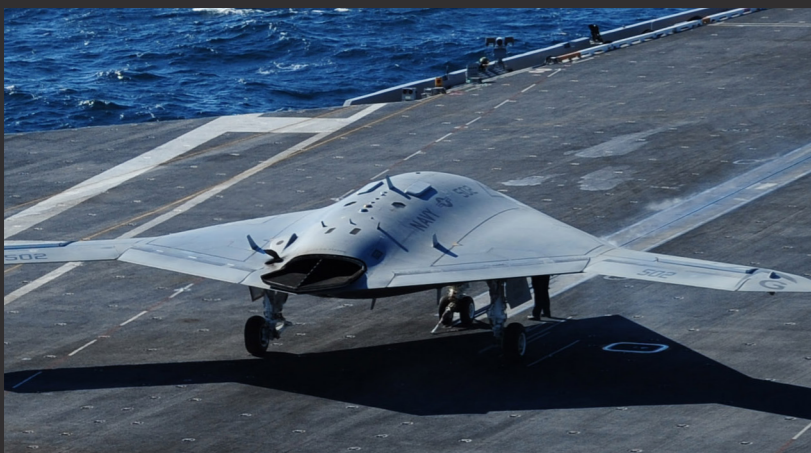
A Navy X-47B Unmanned Combat Air System demonstrator aircraft prepares to execute a touch and go landing on the flight deck of the aircraft carrier USS George H.W. Bush (CVN 77) as the ship conducts flight operations in the Atlantic Ocean on May 17, 2013. This marks the first time any unmanned aircraft has completed a touch and go maneuver at sea. Unmanned aerial vehicles such as the X-47B currently fly in restricted airspace. Efforts are underway to integrate manned and unmanned traffic into the same airspace, but significant human factors challenges must first be addressed.
