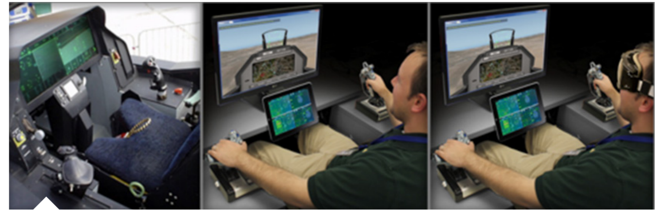
A prototype used for experimentation. These displays use mixed modalities based on ecological interface design techniques.
