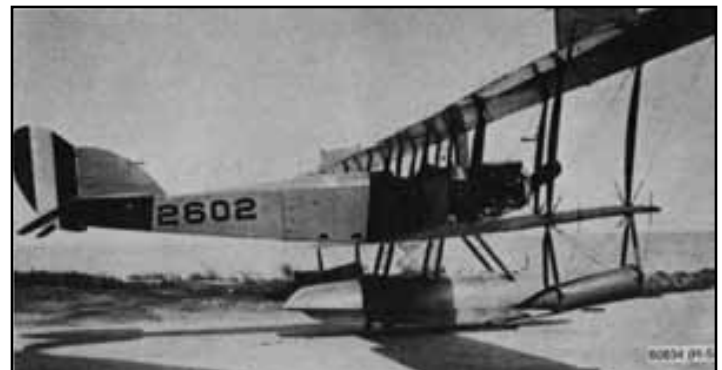
1924 Remote Controlled Pontoon Plane
