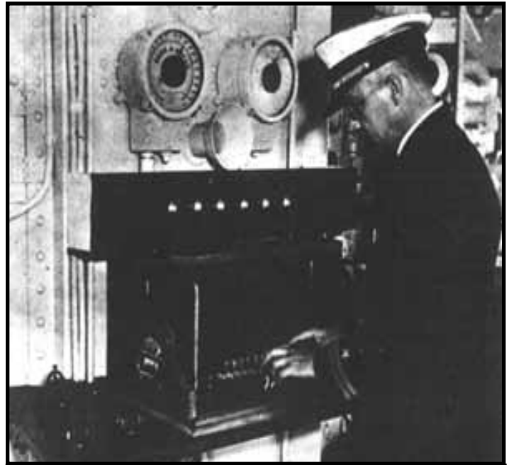
Unidentified officer operating steering and throttle controls of the USS Stodert and USS Utah converted target ships through selector switches based on the teletype mechanisms using the Baudot code.
