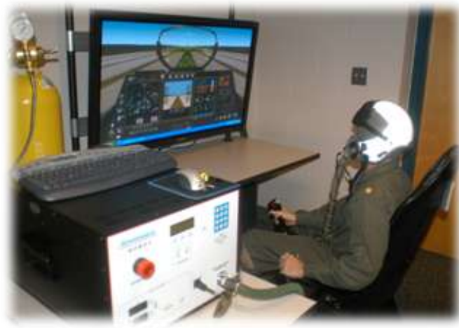
Reduced Oxygen Breathing Device (ROBD) training at the Aviation Survival Training Center simulates an altitude related hypoxia event while students are engaged in a flight simulator task.
